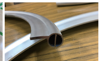
Pipe cross section of a wheel ring
