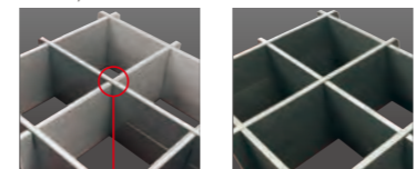
Multi-material basket close-up MAXUS® — for subcriticality Steel — for structural strength Aluminum — for heat transfer
